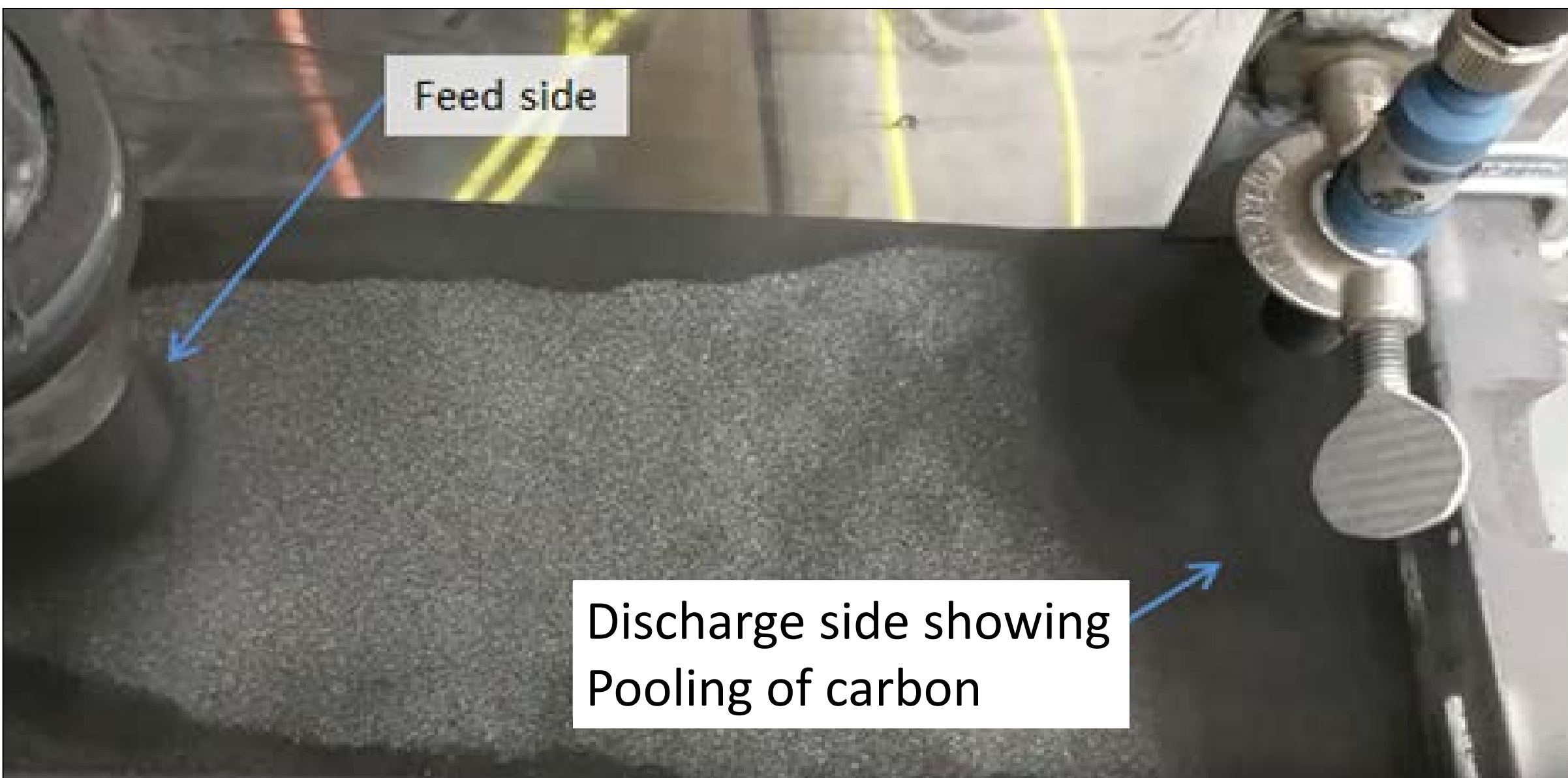
Continuous test of LCS showing large char pooling at bed top
