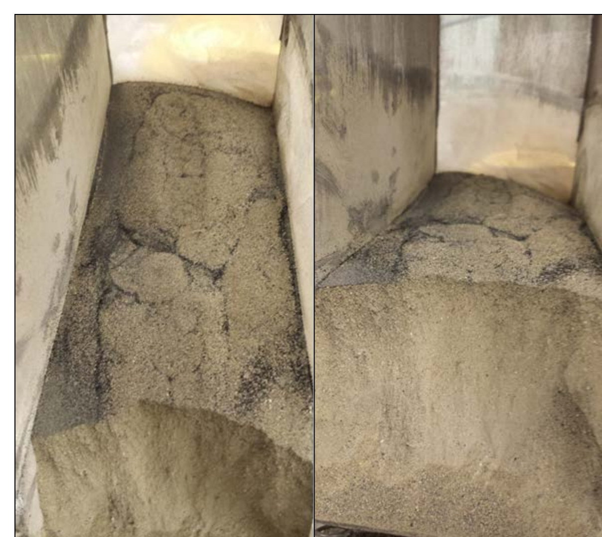
LCS test with GE OC/char mix. Char segregating to top (left); char removal performance for each size bin (right)
